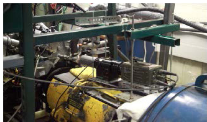
Figure 2. Picture of dyno connected to engine with camera.
